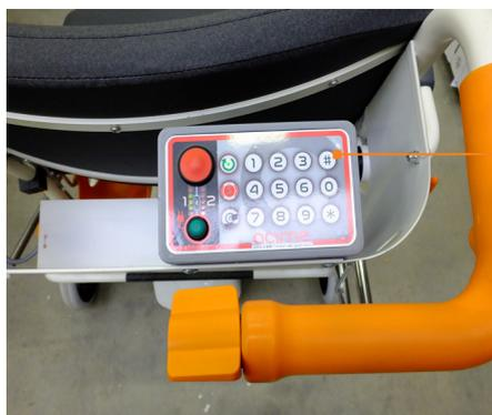
Control panel with safety code and emergency stop integrated.
