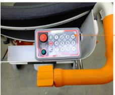
Control panel with safety code and emergency stop integrated.
